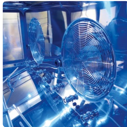
Uniclean® PL II 30 chamber with double H-Flow drying system.
