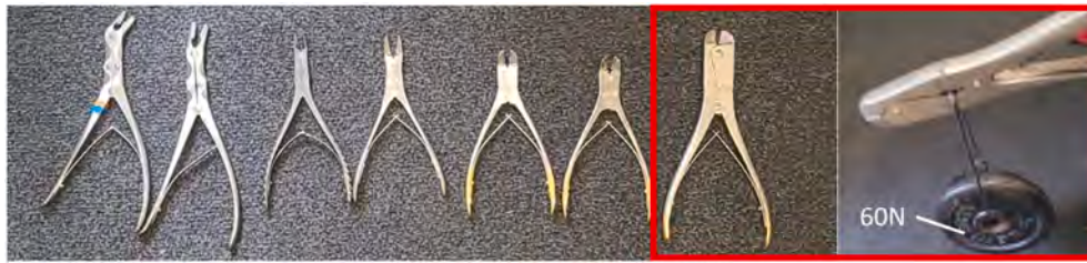
Fig. 4. Testing bone cutting hinge force. Left, tested bone cutters ordered from low to high hinge force. Right, bone cutter with highest hinge force opens when loaded with 6 Kg mass.
